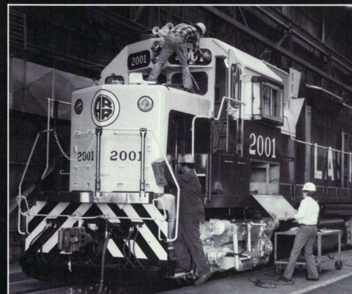
No. 2001 was the first of eight remanufactured 2,000 horsepower locomotives purchased in 1986. The GP38-2s are used in both freight and yard service.
