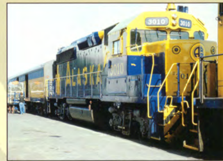
Mechanical Department employees designed an extension to the car body on locomotive No. 3010 and added a head-end power unit. This innovative step improved train efficiency both for winter intermodal service and summer passenger service. All of the work was performed by Alaska Railroad shop crews, despite predictions from other railroads and locomotive manufacturers that the project couldn't be done.
