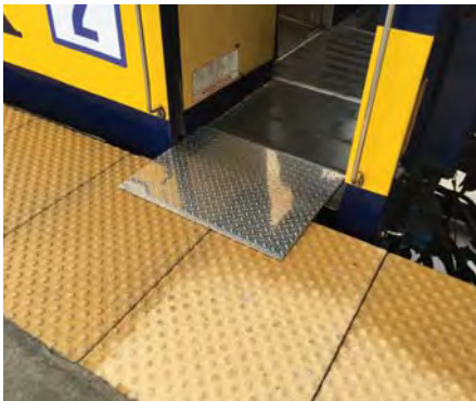
Level Platform Loading Example
