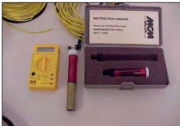
Silver/Silver Chloride Cathodic Protection 1/2 Cell
