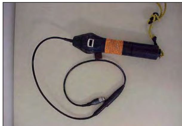
Underwater Ultrasonic Thickness Meter
