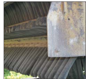
Above top: A ballast regulator is equipped with an arm to scrape vegetation along side the track bed. Above and right: The ballast regulator's bristles are normally covered with rubber, which is stripped to expose the wire when the equipment is used for vegetation management.
