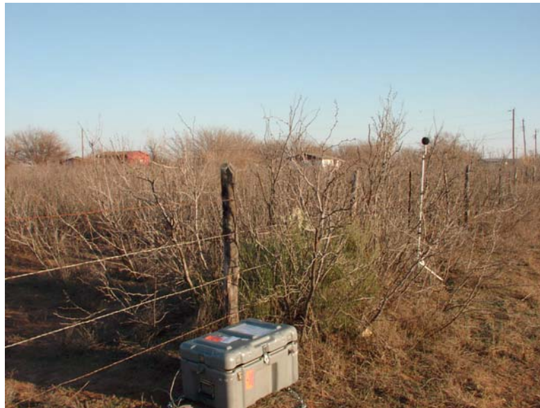
Figure 7. Portable Noise Monitor in Field Application
