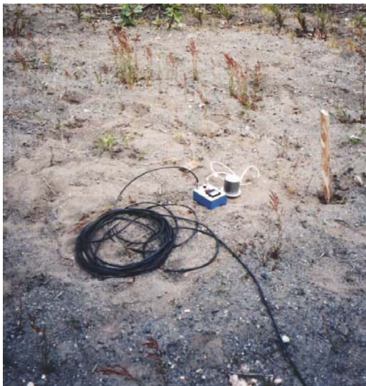
Figure 10. Accelerometer mounted on ground
