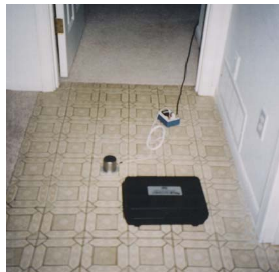
Figure 11. Accelerometer mounted on floor
